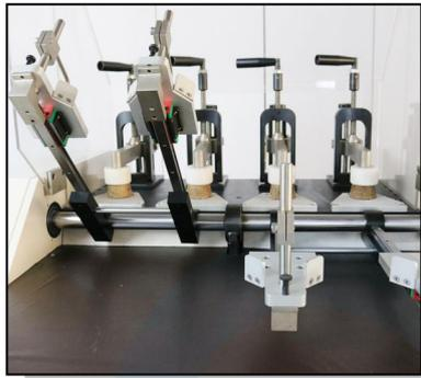
It is to clamp the shoes heel, and release the fix pin when testing to make clamp move freely.
